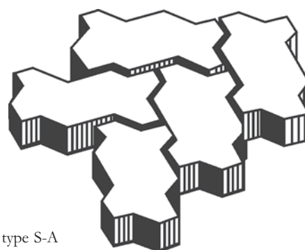
Figure 3a: Type S-A: Those blocks which allow geometrical interlock between all vertical or side faces of adjacent blocks.
