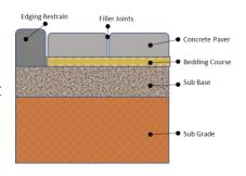
4. **Bedding course:** Sand is used as a bedding course material for paving. The sand must be a well graded, washed river sand or quartize sand. The sand should be between 20mm and 35mm thick and carefully screeded (leveled) with a straight edge prior to placement of the pavers. The sand must be moist
