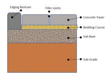
when the pavers are placed. It is not recommended that cement is added to the bedding coarse material.
