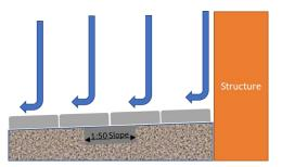
salts to the surface, and thus detract from the appearance and durability of the paving. To create good drainage the sub-grade or excavated surface should have a fall (minimum1:50) so that any moisture will drain to a drainage point. When paving against a building it is recommended that the top of the paving is a minimum of 75mm below the damp proof coarse. It is also advisable to place a plastic membrane against the exposed concrete of the foundation.
