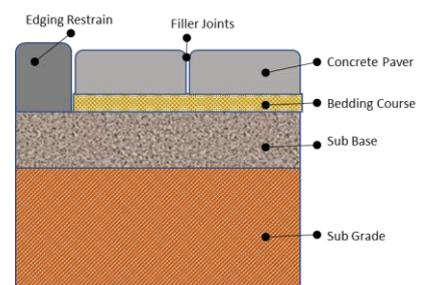
will vary between 50mm and 120mm. In exceptional circumstances, footpath pavers can be laid without a base course where the sub grade material is compact and uniform. The compacted surface should be light or tight or close knit to prevent migration downwards of the bedding course material.
