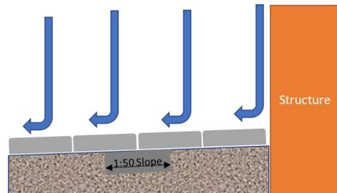
2. **Sub-Grade:** The sub-grade is the upper part of the soil, natural or constructed which supports the loads transmitted by the overlying paving. All vegetation and top soil must be removed. It is advisable to use a weedkiller or geo-textile sheet to prevent weed growth. The sub-grade should be well drained and compact prior to laying the base course material.
