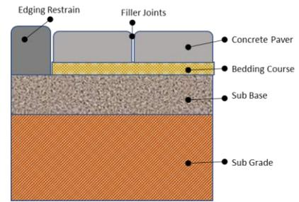
4. **Bedding course:** Sand is used as a bedding course material for paving. The sand must be a well graded, washed river sand or quartzite sand. The sand should be between 20mm and 35mm thick and carefully screeded (leveled) with a straight edge prior to placement of the pavers. The sand must be moist when the pavers are placed. It is recommended that cement is added to the bedding course material to create a firmer base. (1:3 cement/sand ratio).
